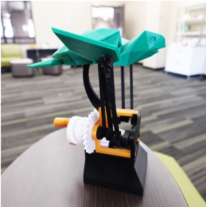
When the orange crank is turned, the 3D-printed sea turtle moves as if swimming.
